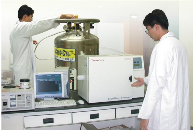
Fig. 5. Programmable cooling freezes samples by gradually cooling them at a controlled rate in a computerized freezer. Photo credit=Chiahsin Lin.
